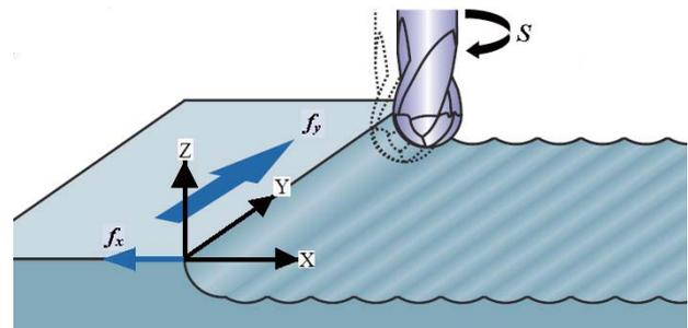
(b) Cutting Tool Movement Direction
