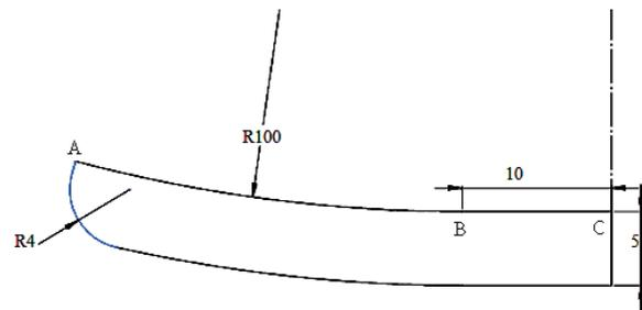
(c) Dimension of the die (Arc AB forms  $15^\circ$  angle at its center)
