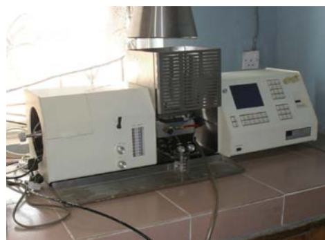
Figure 1 Atomic Absorption Spectrophotometer (AAS) Bulk Scientific Model 210 VGP Used in the Study
