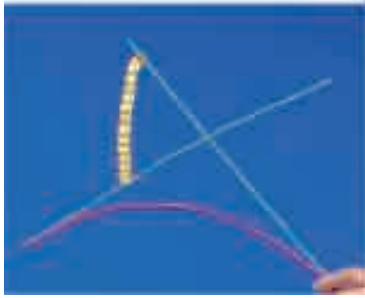
Figure 2 While the tangent angle are the same, the shorter the length of arc, the greater the curving degree
