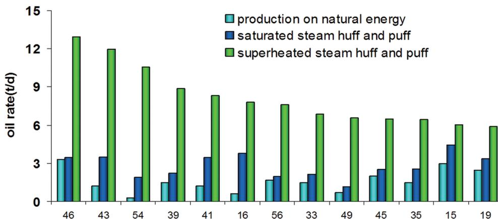
Figure 5 Oil Rate of Single Well Under Three Different Recovery Methods
