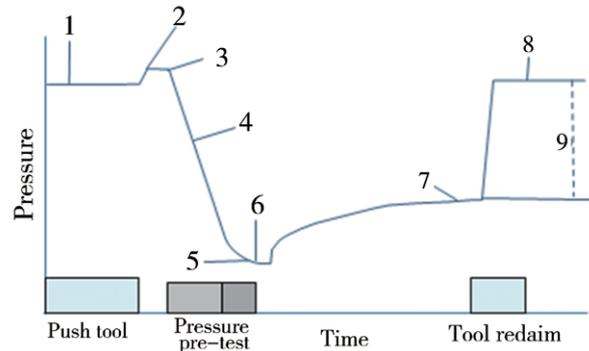
(1- The mud column pressure before testing; 2- The pressure response of the probe to the borehole wall; 3- The pressure starts to fall; 4- Fluid expansion of the tool line; 5- The formation fluid begins to flow into the tool; 6- Pressure starts to recover; 7- Pressure recovers over; 8- The mud column pressure after testing; 9- Wellbore and formation pressure difference)
