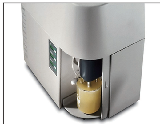
Figure 6 Particle Size Distribution Analyzer (Model MALVERN Mastersizer V2.19)
