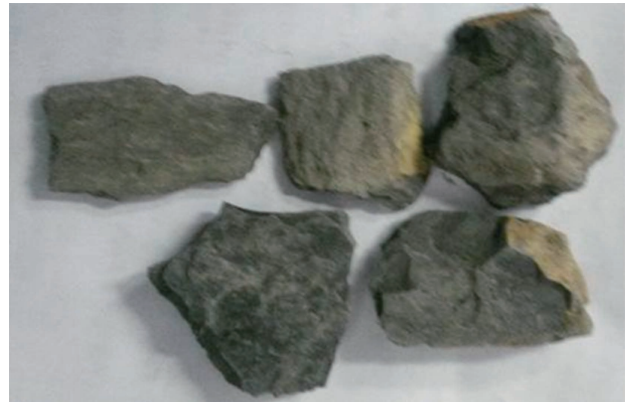
Figure 3 Lower Napo Shale Rock Samples in the COCA Outcrop in the Oriente Basin
