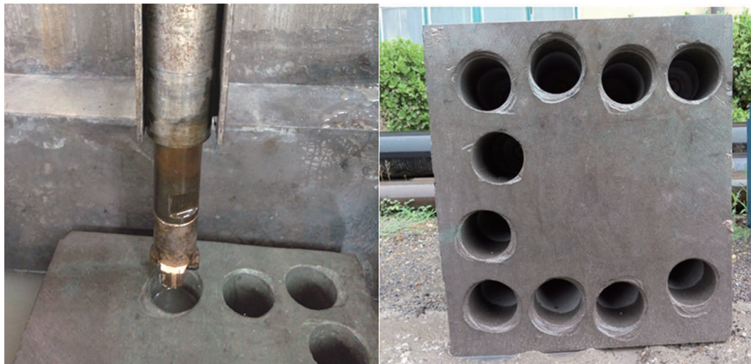
Figure 4 The PDC Drilling Experiments With Rotary Percussion
