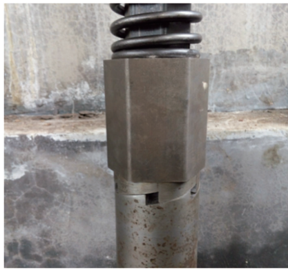
Figure 2 The Structure of Rock Breaking Device With Rotary Percussion
