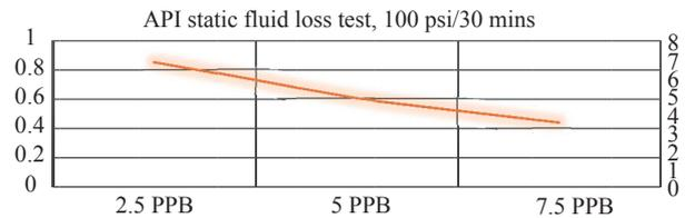
Figure 7 Low Pressure-Low Temperature Static Fluid Loss Test Graphical Result, 100 psi / 30 minutes
