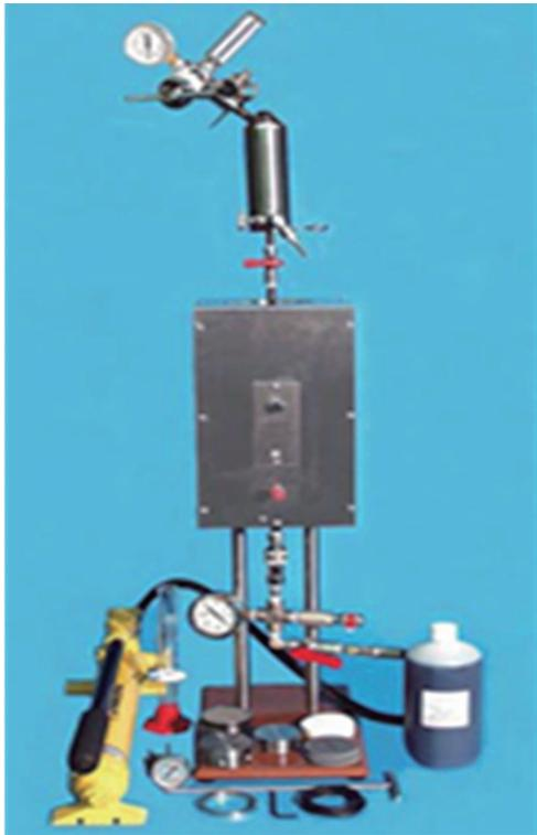
Figure 6 Permeability Plugging Tester
