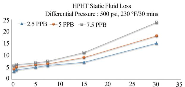
Figure 8 High Pressure-High Temperature Static Fluid Loss Test Graphical Result, Differential Pressure: 500 psi, 230 °F/30 mins
