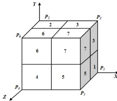
Fig. 1: Illustration of octree nodes distribution
