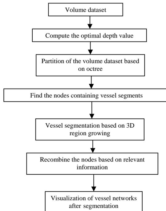
**Fig. 3: Flow diagram of vessel segmentation method**
